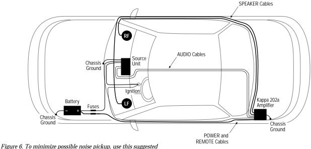
cable routing scheme to plan your amplifier installation.
